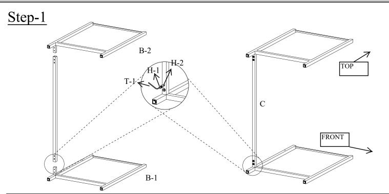
Place the Right Frame (B-1) onto a padded, non-marring surface. Gently insert Stretcher (C) over the corresponding metal post on Right Frame (B-1) as shown, making sure the holes on Stretcher (C) align with the holes on the post. Secure Stretcher (C) using Allen Bolts (H-1) and Flat Washer (H-2). Engage the bolts by hand, but do not fully tighten them yet. Repeat the process above to assemble the Left Frame (B-2) to the other side of Stretcher (C).
