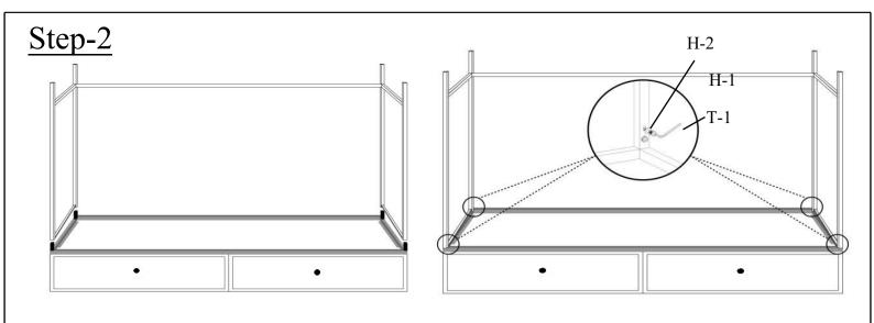
Place the Top (A) upside down on a padded non-marring surface with the help of two people. Place the assembled leg frame onto the underside of the Top (A) ensuring the holes on the Right and Left frame (B-1,B-2) align with the pre-drilled holes on the metal posts of Top (A). Engage the bolts by hand first, and then fully tighten all bolts from Steps 1-2 at this time using Allen Key (T-1).
